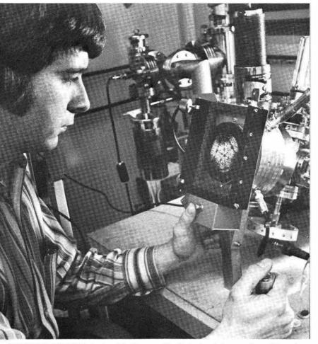
JOHN PANITZ (5114) looks at helium on the first atomic layer of a solid surface through the viewer of a unique new instrument he invented. Called an imaging field desorption mass spectrometer, it was recently patented by ERDA. Bob Crotzer (3646), Foster Tennant (3621) and Jim Taylor (3623) contributed significantly to fabrication of the instrument in the Sandia shops.
